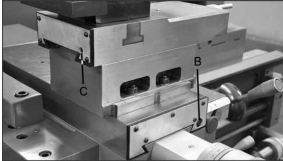
Figure 36 – Gib adjustments, slide and rest
