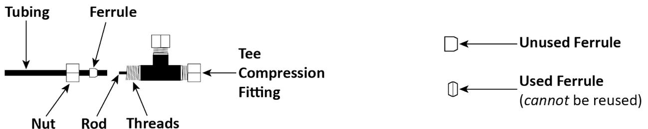
**Important:** ***Ferrules can only be tightened once.*** When you tighten the Nut on the Threads, the Ferrule is compressed; it literally changes shape and ***cannot*** be used again.
