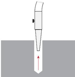
If a vacuum is not available, use a wire brush, hand pump, or compressed air.
