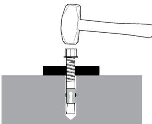
Stop hammering when the washer is snug against the top of the foot.
