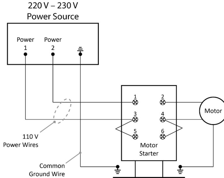
*Motor Starter shown in side view for clarity; the Electrical Box is oriented differently. Not necessarily to scale. Not all components shown.*
