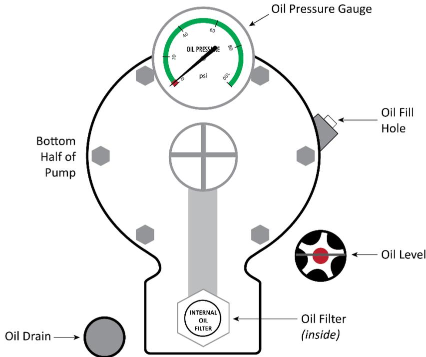
**⚠ WARNING** Do not perform this procedure until a **Planned Shutdown** has been done and you have taken steps to make sure the Compressor cannot be accidentally re-connected to power until you are done with the procedure.
