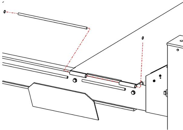
*Drawing shows how to attach the Tire Stop to the front of the Runway.*
