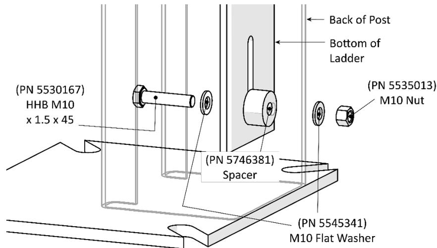
*Front view. Drawing shows the connections to make to the bottom of the Post.*
