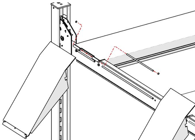
*Drawings shows how to install the Drive-up Ramps at the Drive-up end of the Lift.*
