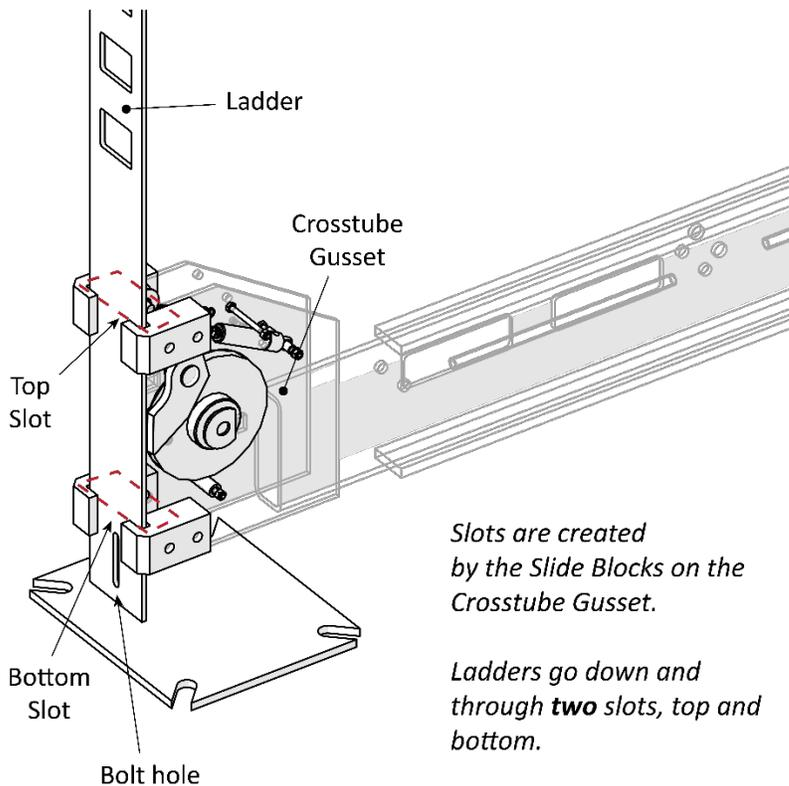
*Drawing shows how to route the Ladders through both Slots created by the Slide Blocks.*
