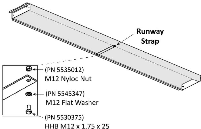
*Drawing shows how to install the Runway Straps to the 3 Offside Runways.*
