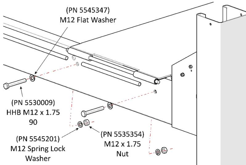
*Drawing shows how to secure the Runways to the Crosstubes.*
