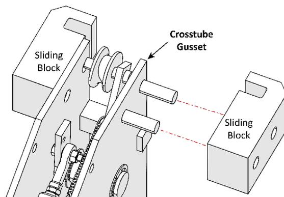
*Top View. Drawing shows how to correctly install two Slide Blocks onto the Crosstube Gusset.*
