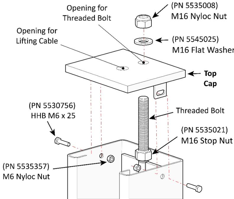
*Drawing shows connections to make to the Top Cap, near the top of the Posts.*
