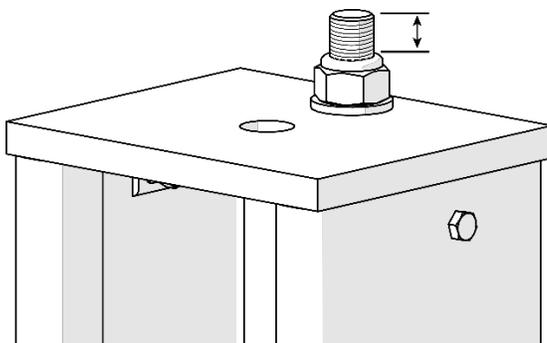
*Drawing shows the threads to leave out above the Top Nut. Adjust as needed.*
