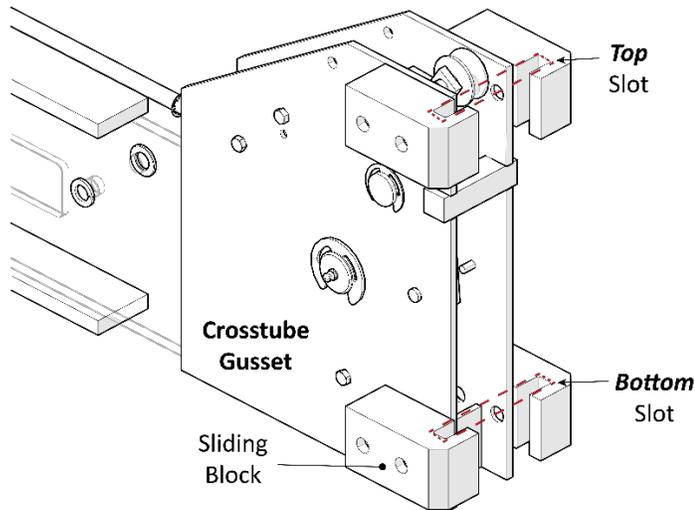
*Front View. Drawing shows the Top and Bottom Slots created by the Slide Blocks.*
