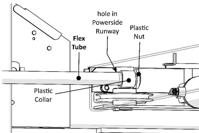
*Drawing shows how to install the Flex Tube to the Powerside Runway.*
