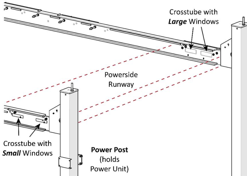
*Top View. Windows are in the Crosstubes; drawing shows how to properly orient the Crosstubes.*
