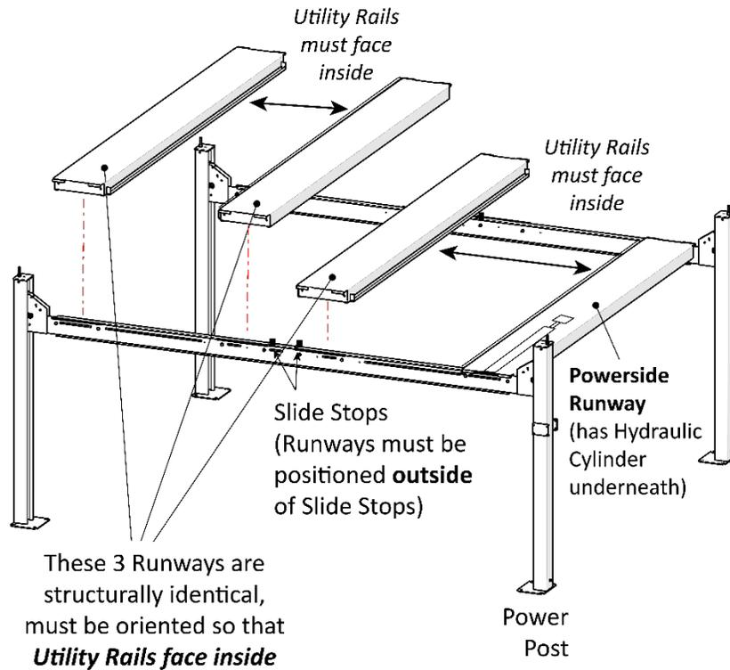
Top View. Cable Sheaves and Hydraulic Cylinder are located on the underside of the Powerside Runway.
