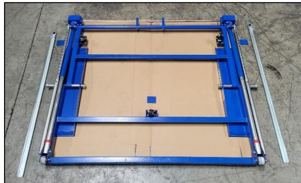
3. (Using the Riser Pads under the Platforms to elevate the lift frame a tad will make this step easier.) Using a Phillips Screwdriver & Wrench or Socket, remove all three Caster Wheels to insert Spacer Plates under each caster base. Retighten Casters & Spacers to lift frame base with same hardware.
