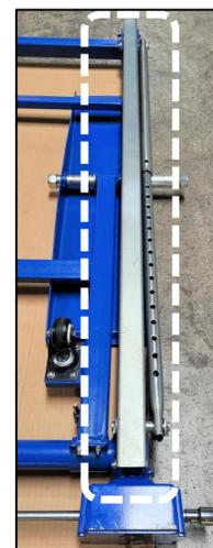
6. Once Floor Rails are installed to the Tilt Lift, carefully flip the Tilt Lift right-side up while lifting from the opposite end of gear boxes. Be sure to hold or secure the loose ends of the Floor Rails while flipping the Tilt Lift back over. Ensure Floor Rails are properly aligned to lift, once flipped right-side up.
