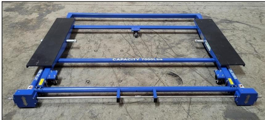
2. Using some form of protection, carefully flip the Lift over onto its topside. Layout Floor Rail parts.
